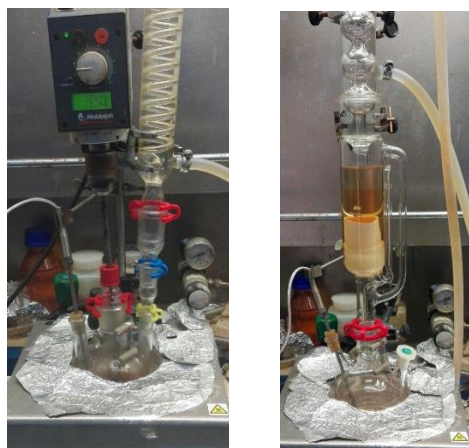
Figure 3 – Experimental set-ups for both synthesis and with the Soxhlet extractor.
